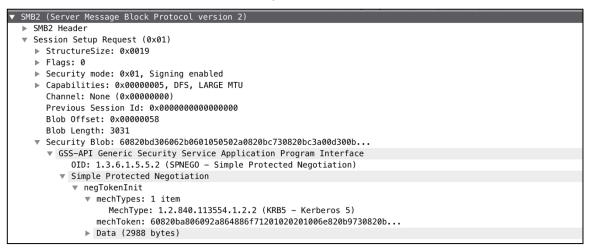
The actual authentication mechanism used is independent of the SMB protocol. It is specified by the GSSAPI and SPNEGO headers. The authentication protocol and data is embedded as an opaque blob into the setup packets. As a matter of practicality, all modern SMB servers support either Kerberos or NTLMSSP or both. Since ConnectedNAS<sup>™</sup> supports both mechanisms, it is able to authenticate with any SMB server.
