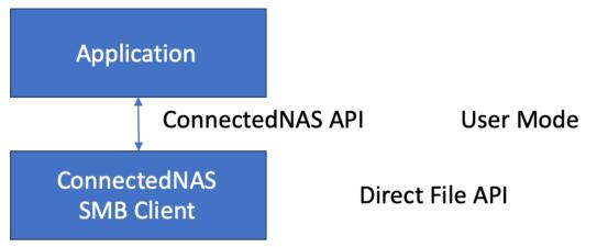
It's a pretty simple model. The Application interacts directly with the SMB Client using the ConnectedNAS<sup>™</sup> API.
